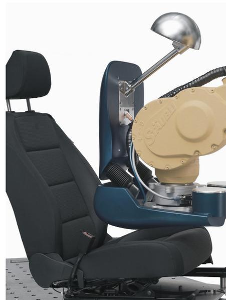
Stäubli robots check the seats at Battenberg.
