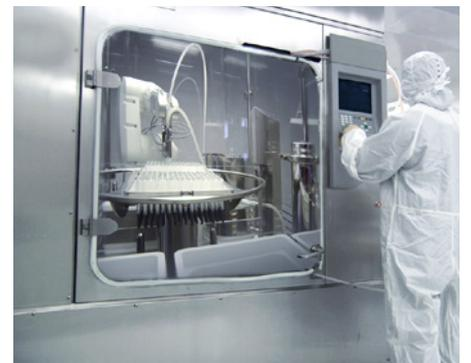
Aseptic isolator with a Staubli Stericlean 6-axis robot arm.
