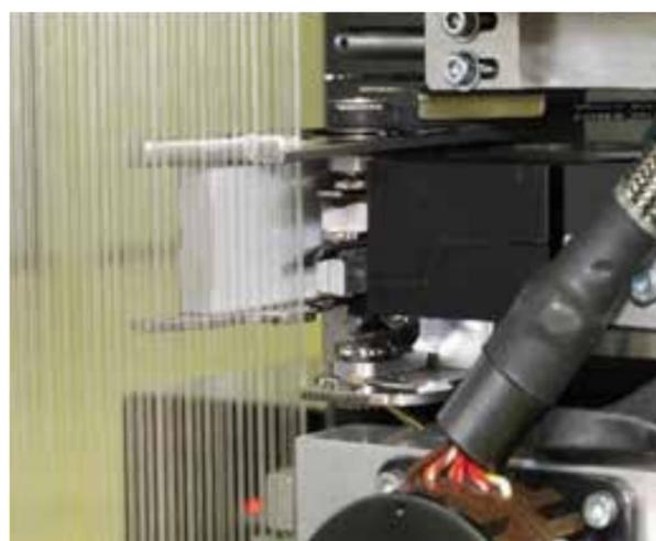
Yarn separation by means of vacuum nozzle
