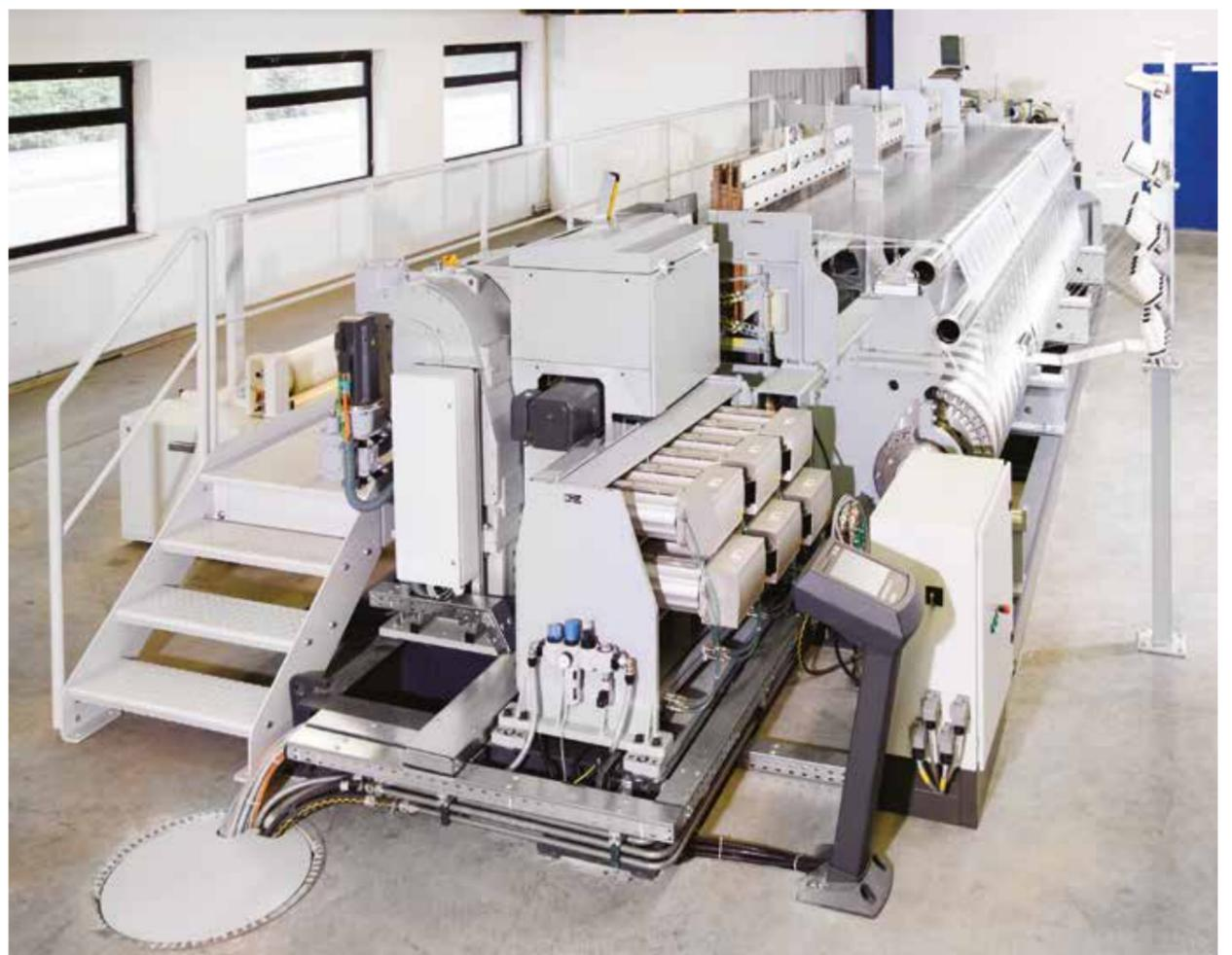
UNIVAL 500T on PMC weaving machine / Foto: courtesy Jürgens Maschinenbau
