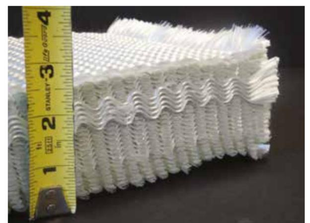
2.7" multilayer fabric made of glass fibre yarns
