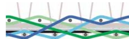
Special ground weave structure for an extra flexible backing fabric (patented)
