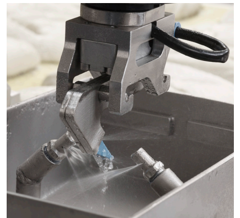
Automated cleaning and moistening of the knife.
