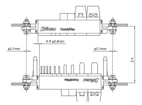
Distance Z in mated condition  $Z = 25 \text{ mm}^{0/+1}$  (with 1.6 mm contacts)  $Z = 25 \text{ mm}^{0/+2}$  (without 1.6 mm contacts)
