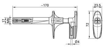
For fast and safe contacting to M6 threaded bolts, for example on motor connections (contact depth 3 to 6 mm). Ø 4 mm rigid socket in handle accepting spring-loaded Ø 4 mm plugs with rigid insulating sleeve. Thread inserts are replaceable and available separately. The current depends on the thread insert.
