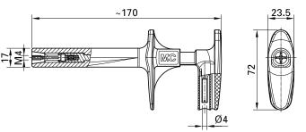
For fast and safe contacting to M4 threaded bolts, for example on motor connections (contact depth 3 to 6 mm). Ø 4 mm rigid socket in handle accepting spring-loaded Ø 4 mm plugs with rigid insulating sleeve. Thread inserts are replaceable and available separately. The current depends on the thread insert.
