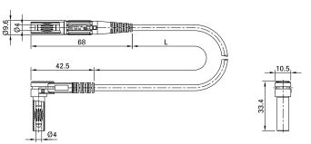
Highly flexible, one end with in-line  $\varnothing$  4 mm MULTILAM plug with rigid insulating sleeve. The other end with right-angled  $\varnothing$  4 mm MULTILAM plug with rigid insulating sleeve.
