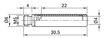
Insulated screw-in adapter with M5 external thread for screw connection to threaded holes. Machined brass. Ø 4 mm rigid socket in insulator accepting spring-loaded Ø 4 mm plugs with rigid insulating sleeve. Socket with internal slot for screwdriver.
