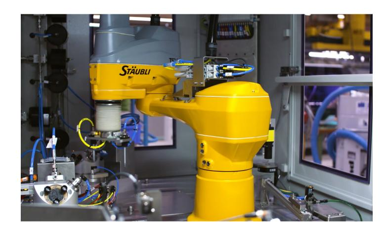
« We wanted a robust robot capable of operating continuously, while ensuring accuracy and repeatability from 2 to 3 hundredths of a millimeter, and fast enough for the client's requested cycle time. Due to small volume of the cell, the very compact TS2-60 robot is ideal for our application »
