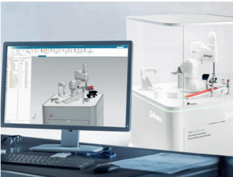
The digital twin is visualised directly next to the real application.
