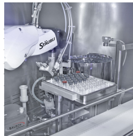
The Stäubli robot precisely stops a tray of nested vials after filling. Changing over seamlessly to different formats, Vers-A-Tech™ can process up to 1,200 nested vials or syringes per hour.
