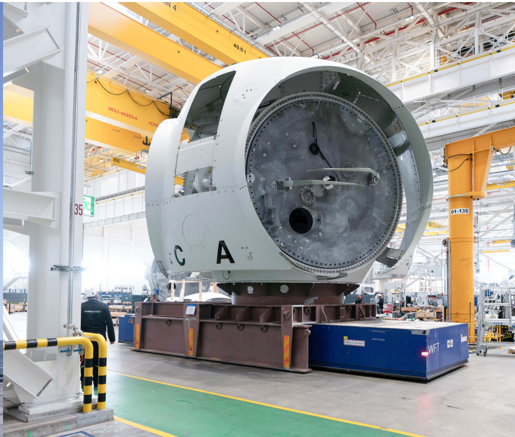
Photo left: Mega dimensions: Two 8MW nacelles present an impressive sight: The frames bearing components weighing many tons are maneuvered by AGV.
