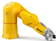
TX2-40/60/90 6 axis robot series with CS9 controller
