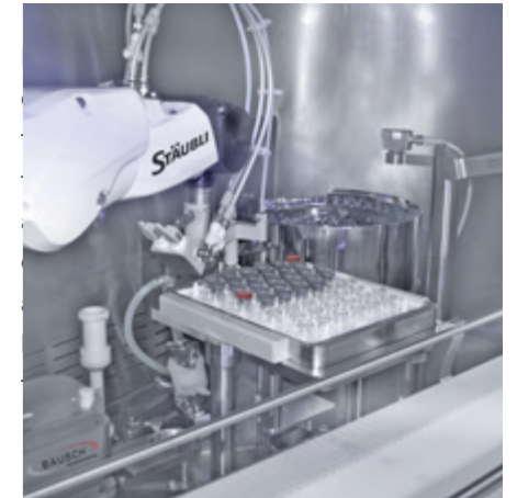
The Stäubli robot precisely stops a tray of nested vials after filling. Changing over seamlessly to different formats, Vers-A-Tech™ can process up to 1,200 nested vials or syringes per hour.
