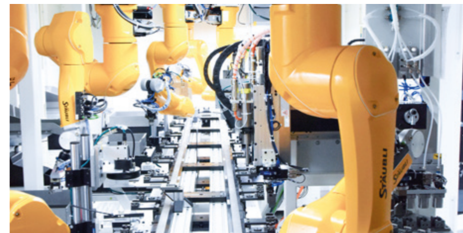
Six ceiling-mounted Stäubli six-axis machines work on the assembly and testing line. Five million high-voltage connectors will be assembled annually on the highly structured assembly line.
