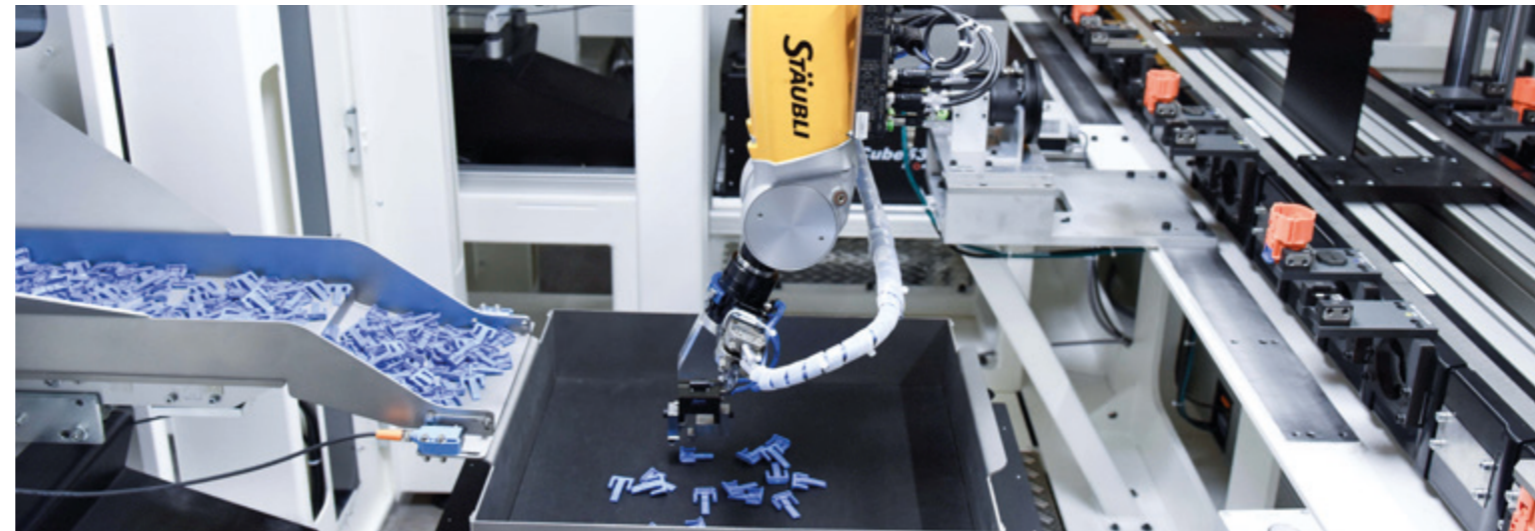
Image left: With its processing head, the robot can complete four welds in a row while in a static state, before repositioning and continuing its works. The Stäubli TX2-90 was the only six-axis robot on the market that was able to meet the requirements in terms of load capacity, range, and precision in such a compact design.
