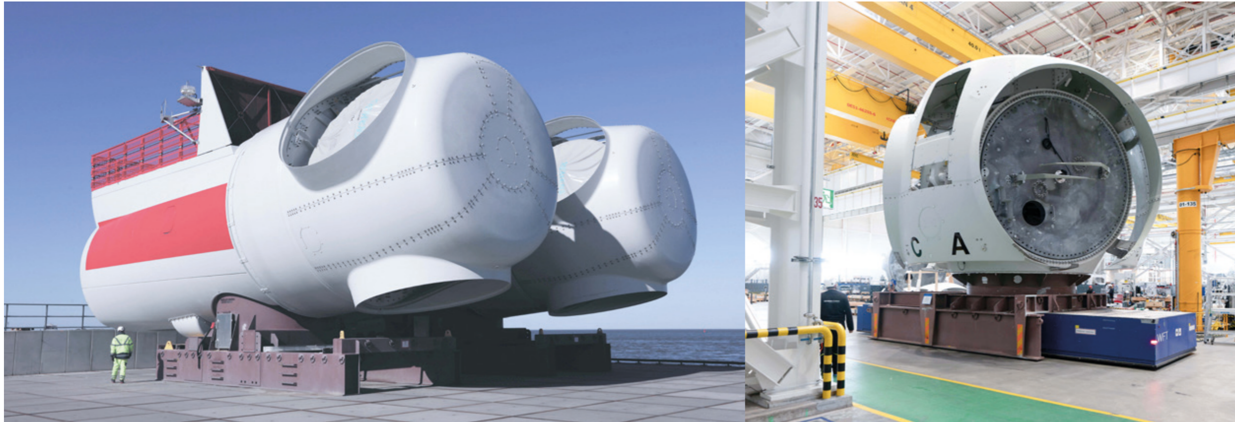
Photo left: Mega dimensions: Two 8MW nacelles present an impressive sight: The frames bearing components weighing many tons are maneuvered by AGV.
