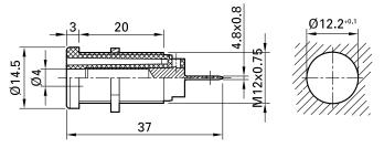
Insulated, rigid, Ø 4 mm, accepting spring-loaded Ø 4 mm plugs with rigid insulating sleeve. Machined brass. The sockets are screwed into predrilled panels of plastic, metal, etc. Flat connecting tab  $4.8~\text{mm} \times 0.8~\text{mm}$ .
