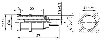
Insulated, rigid,  $\emptyset$  4 mm, accepting spring-loaded  $\emptyset$  4 mm plugs with rigid insulating sleeve. Brass sheet. The socket consists of two insulated, semi-circular contacts, which are connected to each other when a plug is inserted (switch function). The socket is screwed into pre-drilled panels
