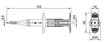
With rigid hook clip made of steel for hooking onto wires.  $\varnothing$  4 mm rigid socket in handle accepting spring-loaded  $\varnothing$  4 mm plugs with rigid insulating sleeve.
