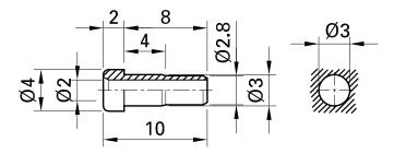
Uninsulated  $\varnothing$  2 mm rigid. Machined brass. The socket is soldered into predrilled panels.
