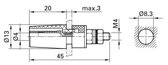
Insulated, rigid, Ø 4 mm, accepting spring-loaded Ø 4 mm plugs with rigid insulating sleeve. Machined brass. The socket is surface-mounted in pre-drilled panels of plastic, metal, etc. Threaded bolt M4.
