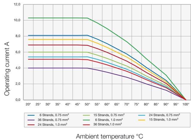
**NBR/CR: Cable 1.5 mm<sup>2</sup>**
