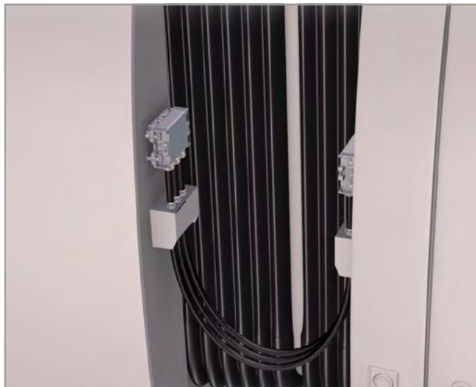
Examples of intercar couplings with straight and right-angled EvoTrak MPC plug combinations. Even three-level solutions are possible.
