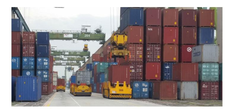
In 2040 when PSA Singapore's Tuas Mega Port is fully operational, it will be the world's largest fully automated container terminal in a single location. In preparation for this new mega port, automated charging systems for a fleet of battery-powered automated guided vehicles (AGVs) with a carrying capacity of 65 tonnes and a cruising speed of 25 km/h were tested and evaluated.
