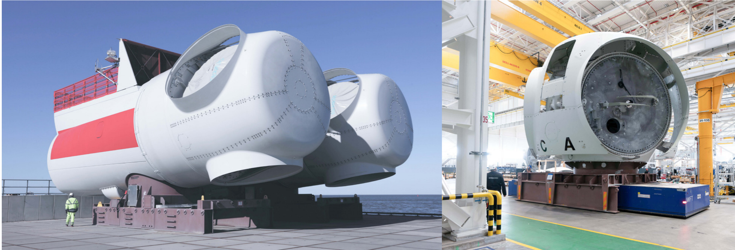
Photo left: Mega dimensions: Two 8MW nacelles present an impressive sight: The frames bearing components weighing many tons are maneuvered by AGV.
